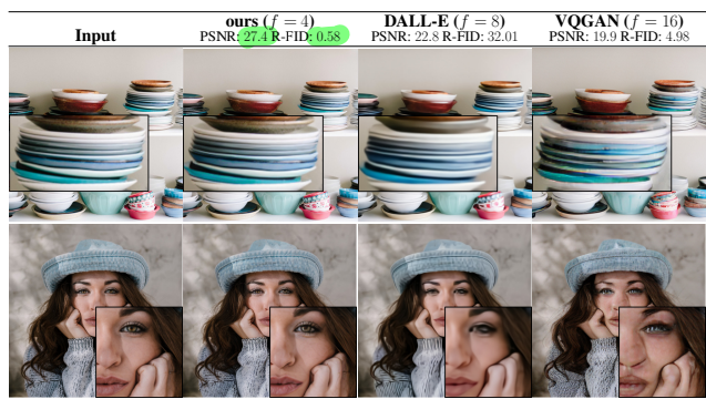
Figure 1. Boosting the upper bound on achievable quality with less aggressive downsampling . Since diffusion models offer excellent inductive biases for spatial data , we do not need the heavy spatial downsampling of related generative models in latent space, but can still greatly reduce the dimensionality of the data via suitable autoencoding models, see Sec. 3. Images are from the DIV2K [1] validation set, evaluated at 512^2 px. We denote the spatial downsampling factor by f . Reconstruction FIDs [29] and PSNR are calculated on ImageNet-val. [12]; see also Tab. 8.
